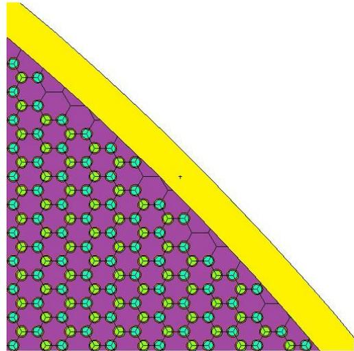
Fig. 3. The MCNP model of one core region showing the radial layout of the different materials in the core with Hastelloy-N (orange clad or yellow vessel), hot and cold FLiBe (light green and blue respectively) and fuel (purple).
