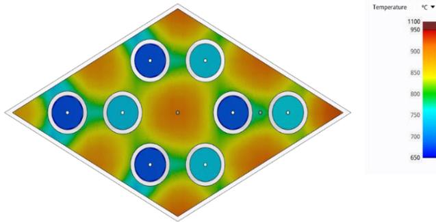
Fig. 4. Color map of the horizontal cross section of the single channel temperature model.
