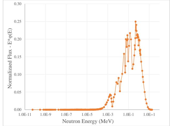
Fig. 4. In-core average neutron flux spectrum of the U-tube Stationary Salt Reactor.
