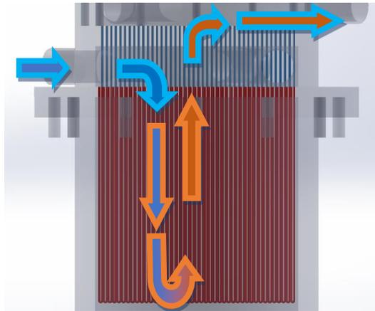
Fig. 2. Side view of the SOLIDWORKS model with flow path arrows.
