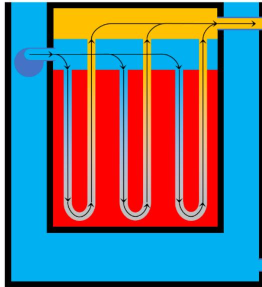
Fig. 1. A reactor diagram illustrating coolant flows (not to scale). Blue to orange gradient represents the cold to hot gradient of the FLiBe coolant, and red is fuel.
