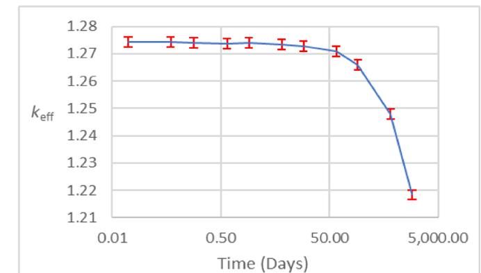
Fig 3. Subassembly  $k_{eff}$  as a function of burnup.
