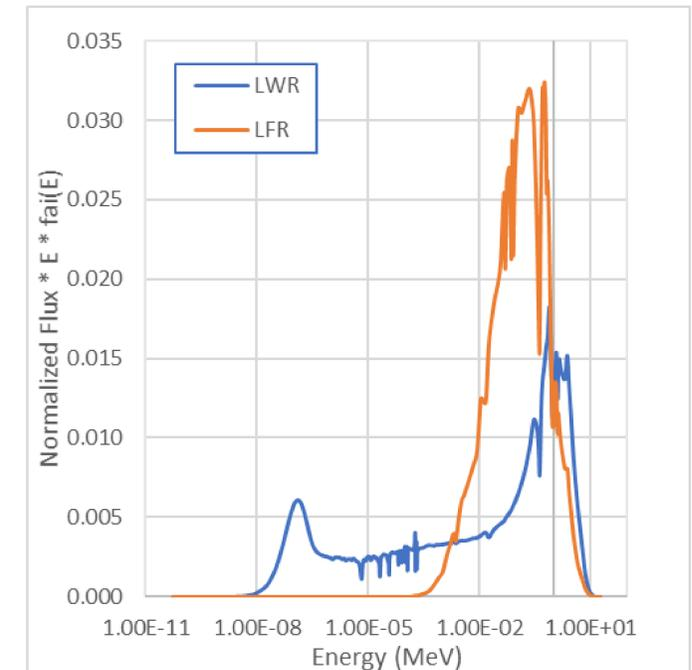
Fig 2. Flux spectrum comparison between a typical LWR and the LFR reactor.
