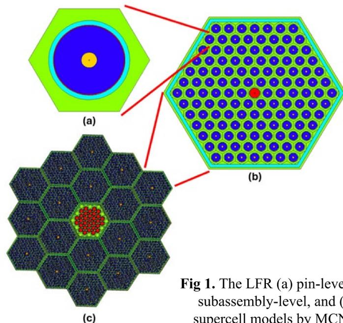
Fig 1. The LFR (a) pin-level, (b) subassembly-level, and (c) supercell models by MCNP.
