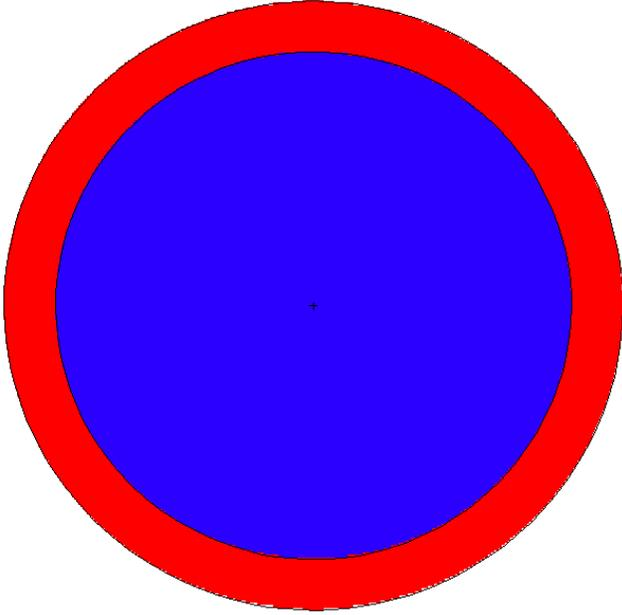
Figure 2. 2-D view of the homogeneous fuel pebble in the Xe-100 reactor. From inside to out the layers are: homogenized TRISO particle carbon matrix material (blue), outer carbon layer (red).
