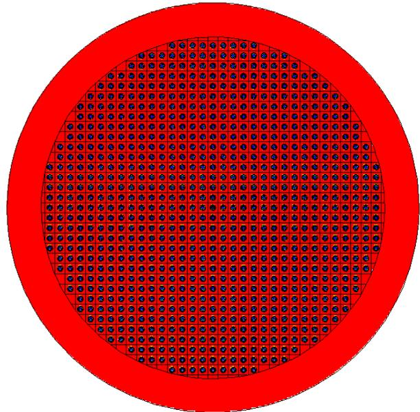
Figure 3. 2-D view of the heterogeneous (unclipped) pebble model in the Xe-100 reactor. Carbon matrix material (red), heterogeneous TRISO particles (blue spheres).
