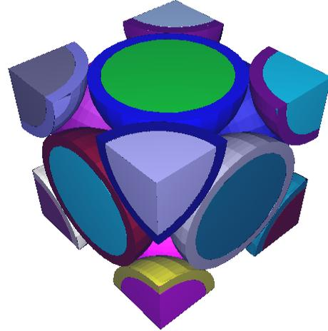
Figure 5. 3-D view of the FCC homogeneous pebble model with helium in the Xe-100 reactor.
