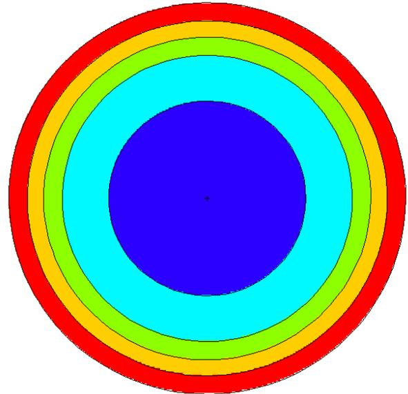
Figure 1. 2-D view of the TRISO fuel particle in the Xe-100 reactor. From inside to out the layers are: fuel kernel (blue), porous carbon (cyan), inner pyrolytic carbon (green), silicon carbide (orange), outer pyrolytic carbon (red).
