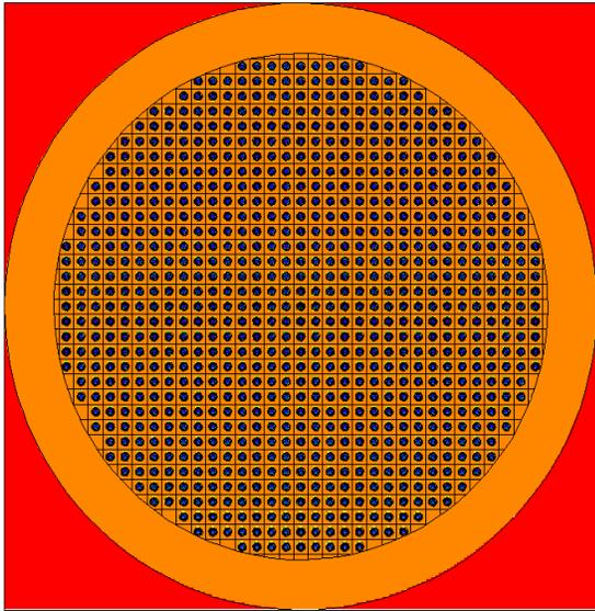
Figure 4. 2-D view of the unclipped heterogeneous pebble model with helium in the Xe-100 reactor. Carbon matrix material (orange), heterogeneous TRISO particles (blue spheres), helium (red).
