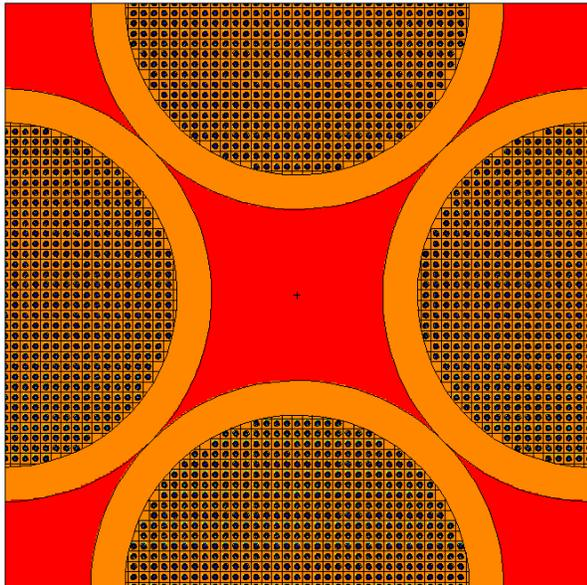
Figure 7. 2-D view of the FCC heterogeneous semi-unclipped pebble model with helium in the Xe-100 reactor.
