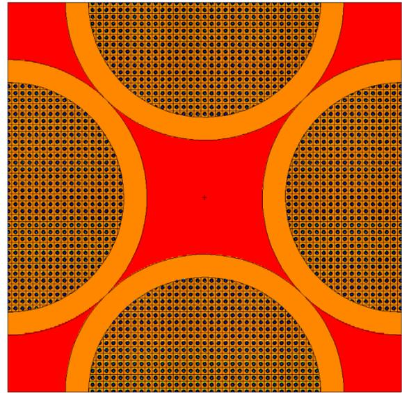
Figure 6. 2-D view of the FCC heterogeneous pebble model with helium in the Xe-100 reactor. Carbon matrix material (orange), heterogeneous TRISO particles (blue spheres), helium (red).
