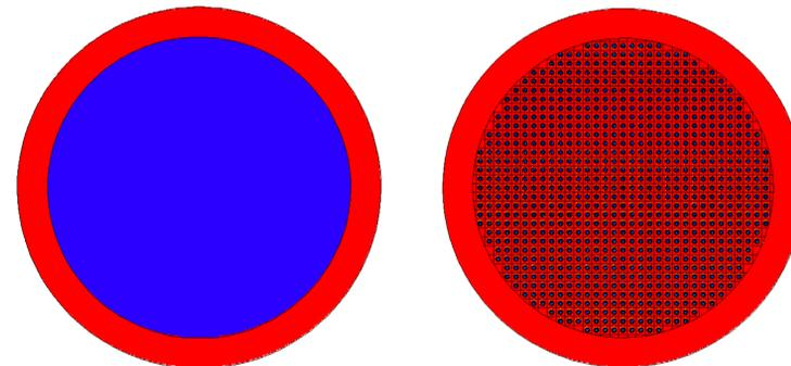
Figure 2. The 2-D view of the homogeneous (left) and unclipped heterogeneous (right) fuel pebble in the Xe-100 reactor. For the homogenous model, from inside to out the layers are: homogenized TRISO particle carbon matrix material (blue), outer carbon layer (red); for the heterogeneous model, the carbon matrix material is shown in red and heterogeneous TRISO particles are shown as small blue spheres.
