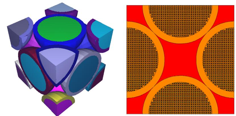
Figure 3. The 3-D (left) and 2-D (right) view of the FCC homogeneous pebble model with helium (red) and graphite (orange) in the Xe-100 reactor.
