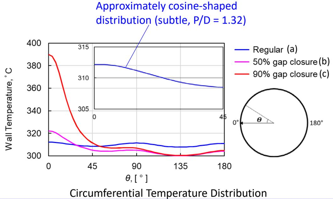
*As the rod displaces towards its neighboring rod, temperature increases at the gap closure side, while decreases at the opposite side, forming a thermal gradient in the transverse direction that leads to further deformation.*
