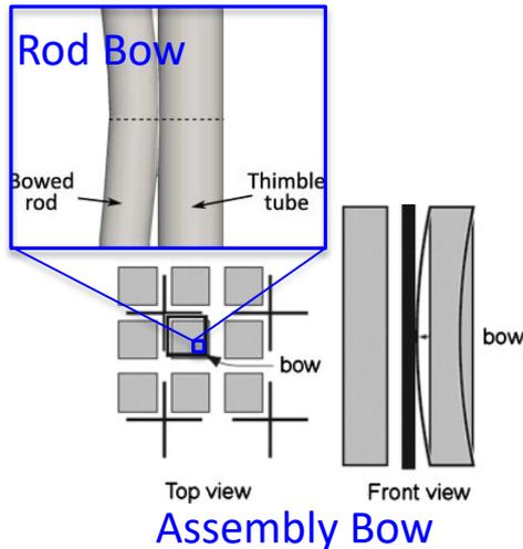
Schematic illustration of fuel rod and assembly bowing.
