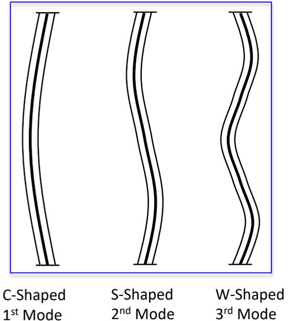
A Schematic Illustration of Fuel Rod and Fuel Assembly Bowing Configuration
