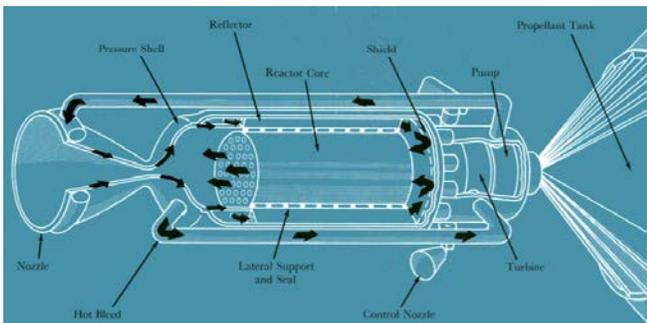
**Figure 3.** Shows the inside of the NERVA rocket [2].
