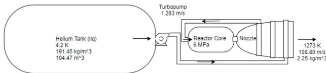
**Figure 4.** Propellant Flow Diagram.
