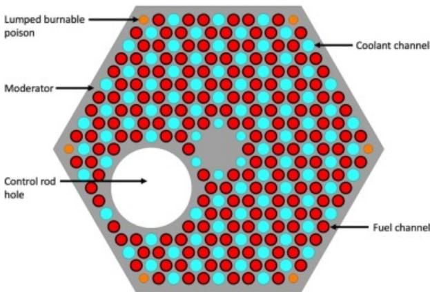
**Figure 2.** Cross-Section of a Single Fuel Block [3].
