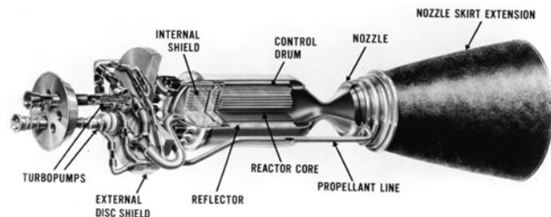
**Figure 1.** NASA NERVA Project Schematic [1].
