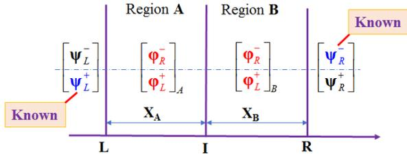
**Figure 2.** Configuration for a two-region problem in slab.
