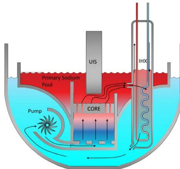
**Figure 1: A schematic of thermal stratification that can exist in the reactor pool in the event of a reactor trip (Blue represents colder sodium and red represents hotter sodium; black arrows show the flow path of the primary coolant).**
