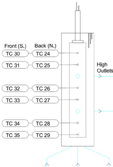
**Figure 5: Layout of thermocouple location inside of the test section.**
