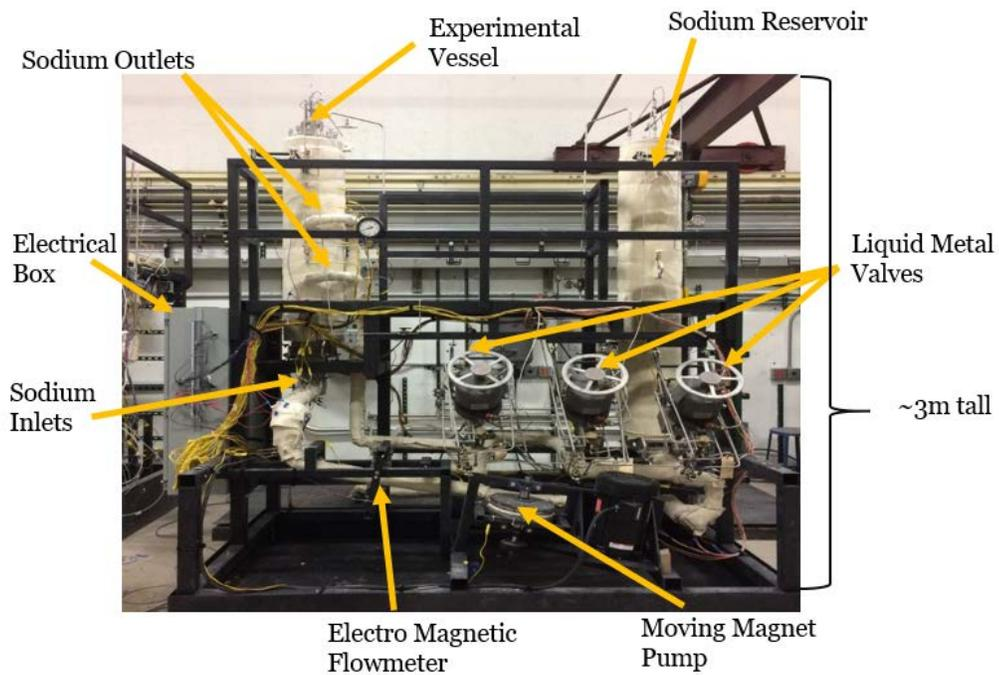
**Figure 3: Thermal Stratification Testing Facility as of May 2018.**
