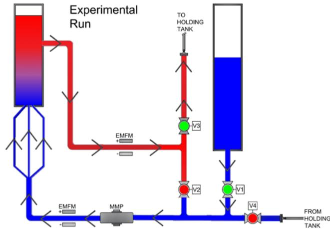
**Figure 4: Operation of the TSTF during an experimental run.**
