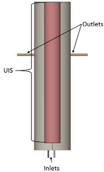
**Fig. 2. Test Section inside of the TSTF.**
