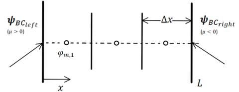
Fig.1. 1D transport mesh scheme with boundary conditions.
