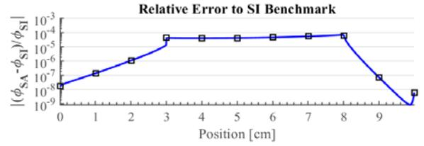
Fig. 4. Heterogenous slab case semi-log relative error.
