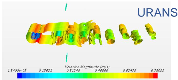
Turbulent mixing in a T-junction
