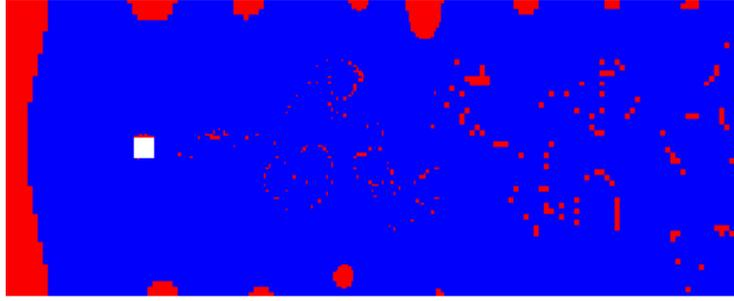
Flow past a square cylinder with symmetry boundaries on the top and bottom, activation regions of the original STRUCT model (in blue)
