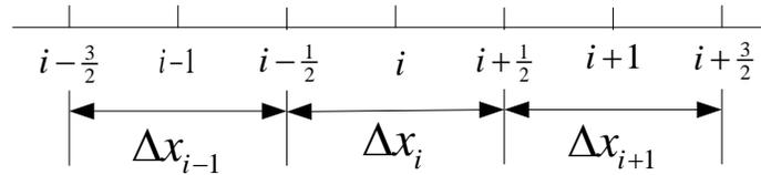
**Figure 1.** Spatial discretization configuration for the slab geometry.
