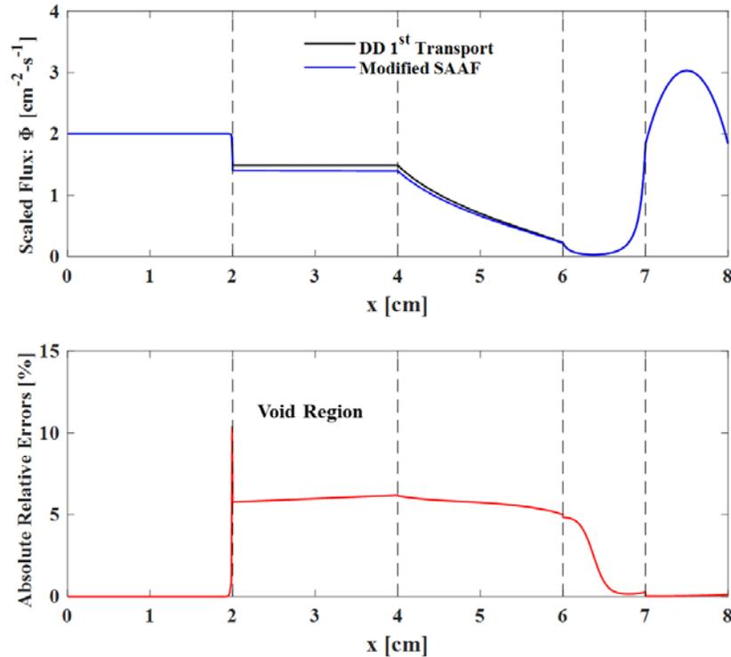
**Figure 5.** Comparison of the scale flux distribution solution for Prob. 2 obtained by the DD method on standard 1<sup>st</sup> order transport equation and the standard CFEM method on modified SAAF equation.
