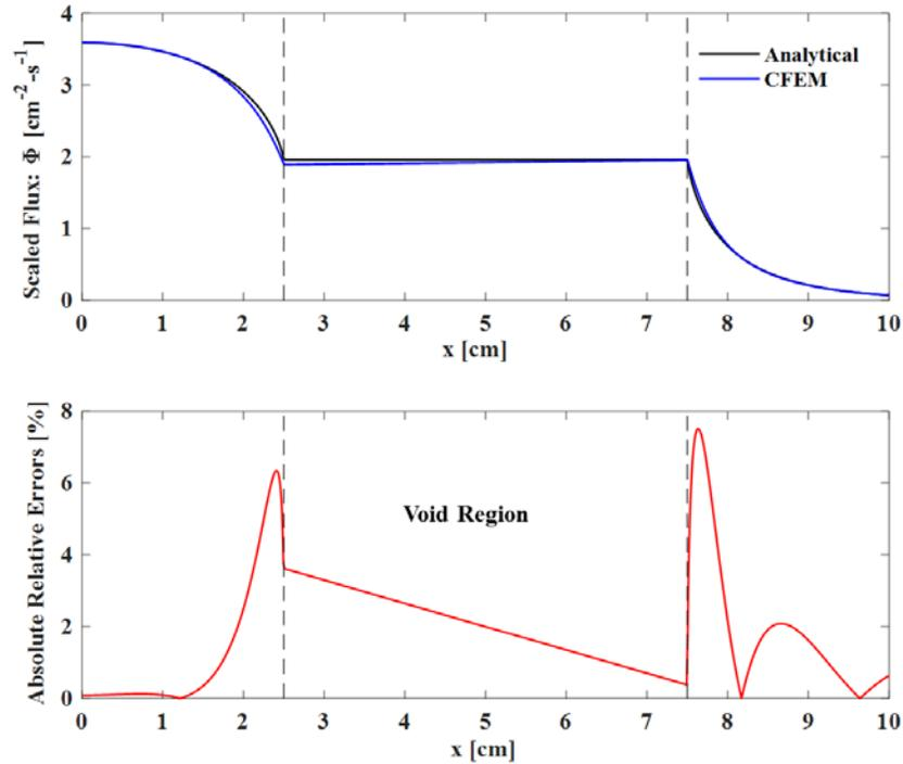
**Figure 4.** Comparison of the scale flux distribution solution for Prob.1 obtained by the analytical method and the standard CFEM method on modified SAAF equation.
