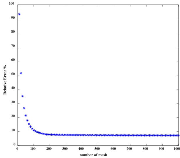
**Figure 2.** Relative error (%) and different number of mesh for regions 1 to 3 at Prob. 1.
