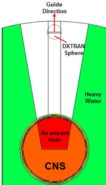
**Figure 3.** An illustration of the MCNP tally performed for the CNS brightness calculation.
