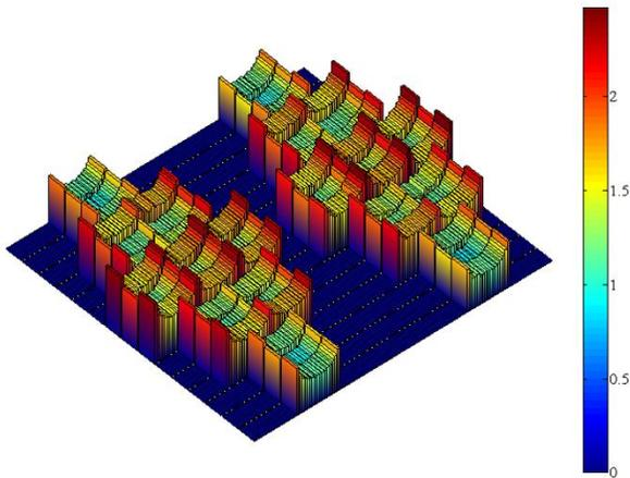
**Figure 2.** Power distribution at the mid-plane of the SU core.
