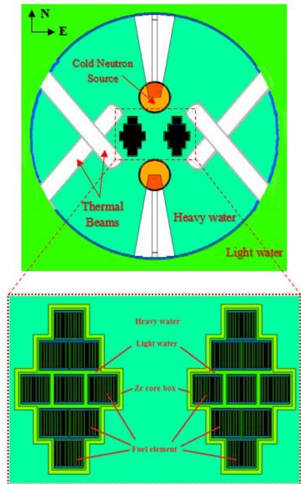
**Figure 1.** A schematic view of the mid-plane of the reactor with horizontally split cores
