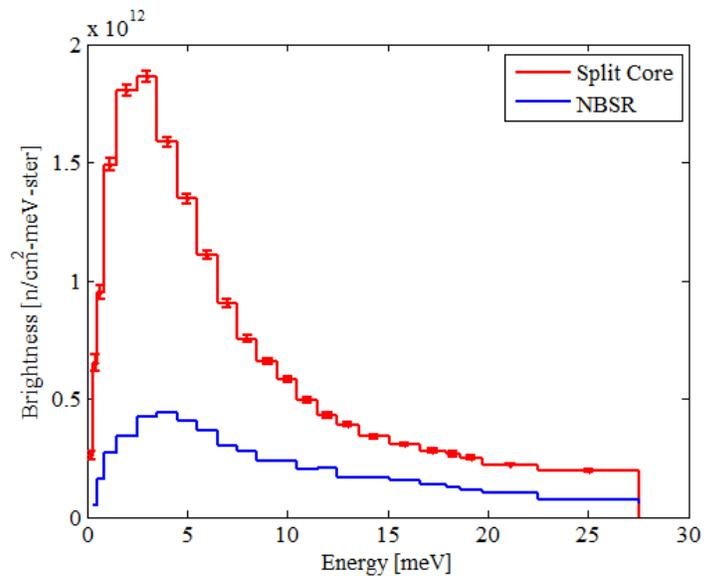
**Figure 4.** The comparison of CN brightness in the split core to that at NBSR.
