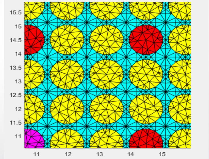
magnified view of the unstructured meshes of the UO<sub>2</sub> assembly (units: cm)
