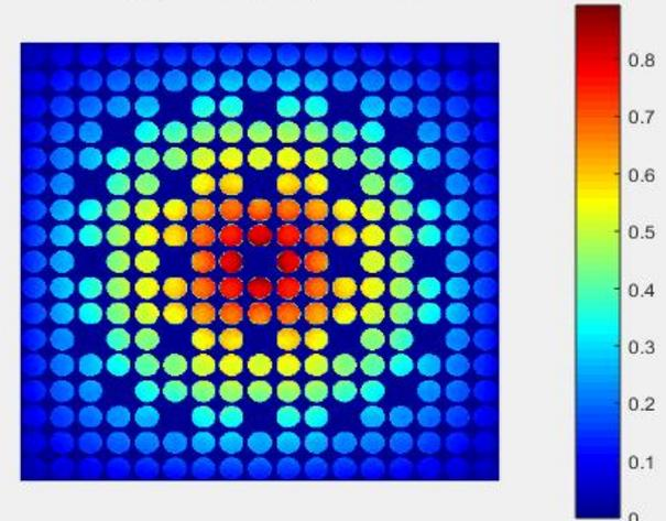
Fission reaction rate profile (UO<sub>2</sub> assembly)
