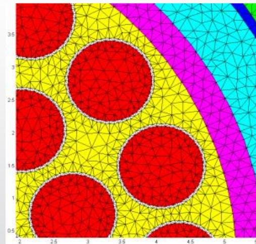
A magnified view of the unstructured meshing of a CANDU fuel bundle [6]
