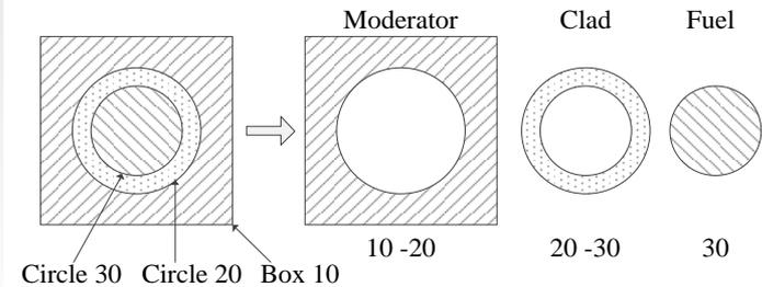
A unit cell composed by three CSG objects [6]
