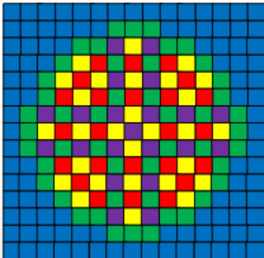
Legend:- yellow: controlled MOX assembly (24); purple: controlled  $\text{UO}_2$  assembly (21); red: uncontrolled MOX assembly (28); green: uncontrolled  $\text{UO}_2$  assembly (48).
